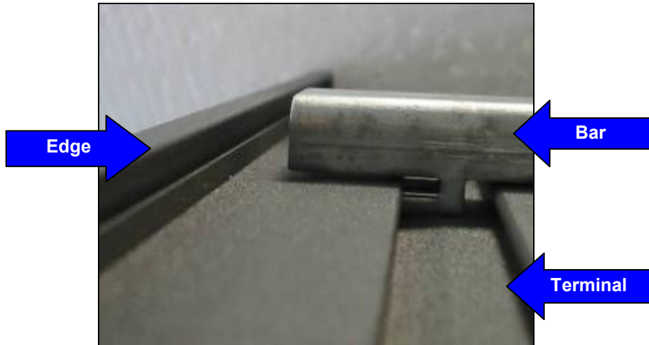
Figure 4-6: Profile of fixing tool.
